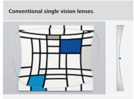
Conventional designs lead to distortions in the lens periphery.
